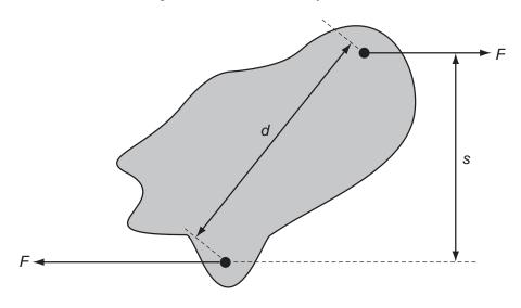
What is the magnitude of the torque on the body produced by these forces?
